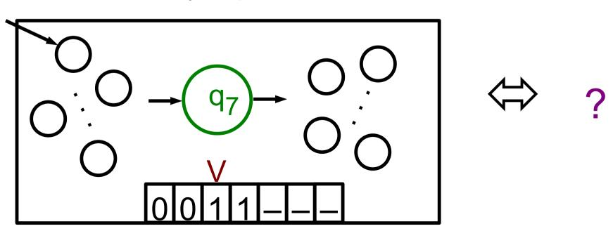
Definition: A configuration of a TM specifies contents of tape, state, head location
