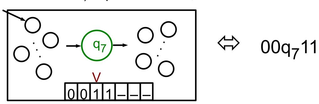
Definition: A configuration C yields a configuration C' if TM goes from C to C' in one step:
