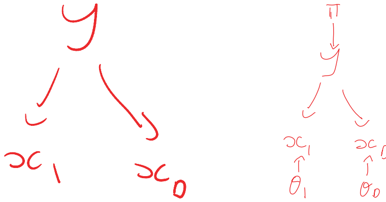
Figure 4: Naive Bayes classifier represented as a DGM. y is the class label and x_i are the features. In the version on the right, the parameters are shown explicitly.
