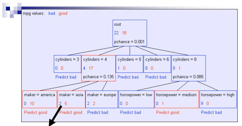
Recursively build a tree from the seven records in which there are four cylinders and the maker was based in Asia
