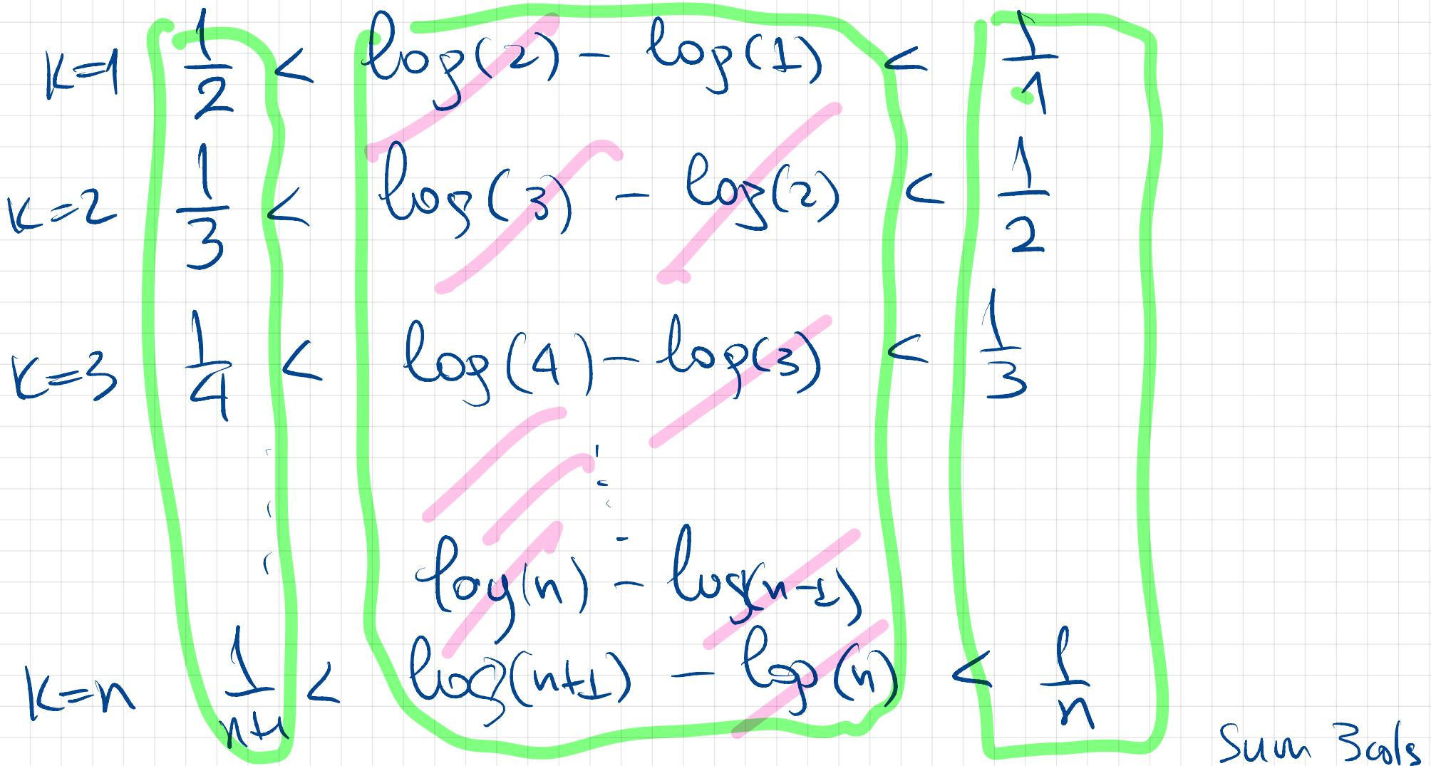
$$\frac{1}{2} + \frac{1}{3} + \dots + \frac{1}{n+1} < \log(n+1) - \log(1) < \frac{1}{1} + \frac{1}{2} + \dots + \frac{1}{n}$$
