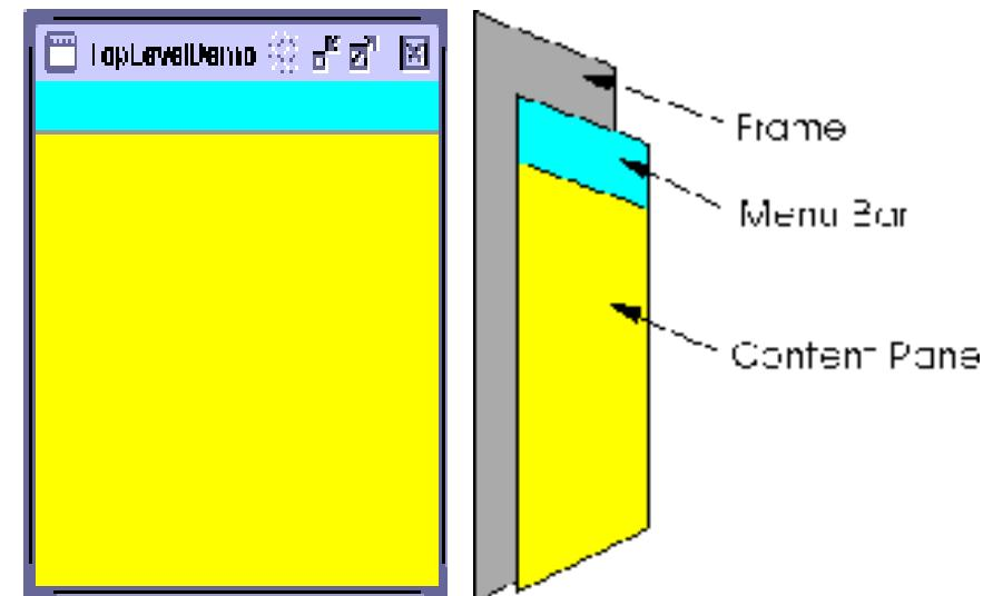
As a rule, a standalone application with a Swing-based GUI has at least one containment hierarchy with a **JFrame** as its root
