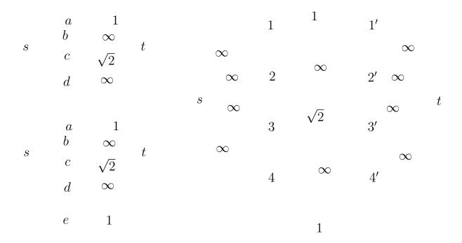
Figure 1: A pathological example for the basic augmenting path algorithm.
