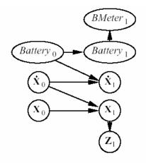
Modeling a robot with position sensors and a battery charge meter
