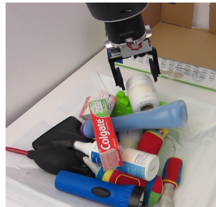
Figure 1. The grasp detection methods proposed in this paper enable us to obtain high grasp success rates in dense clutter such as that shown here.
