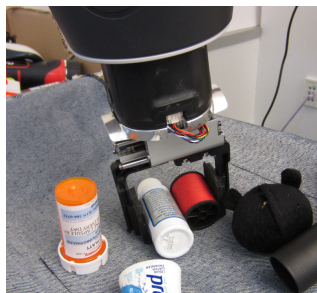
Figure 16. One grasp detection failure mode: two objects are grasped as if they were a single object.
