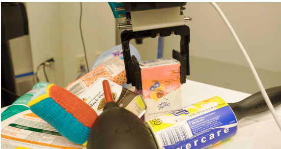
Figure 13. Gripper closing on the first object in the clutter.
