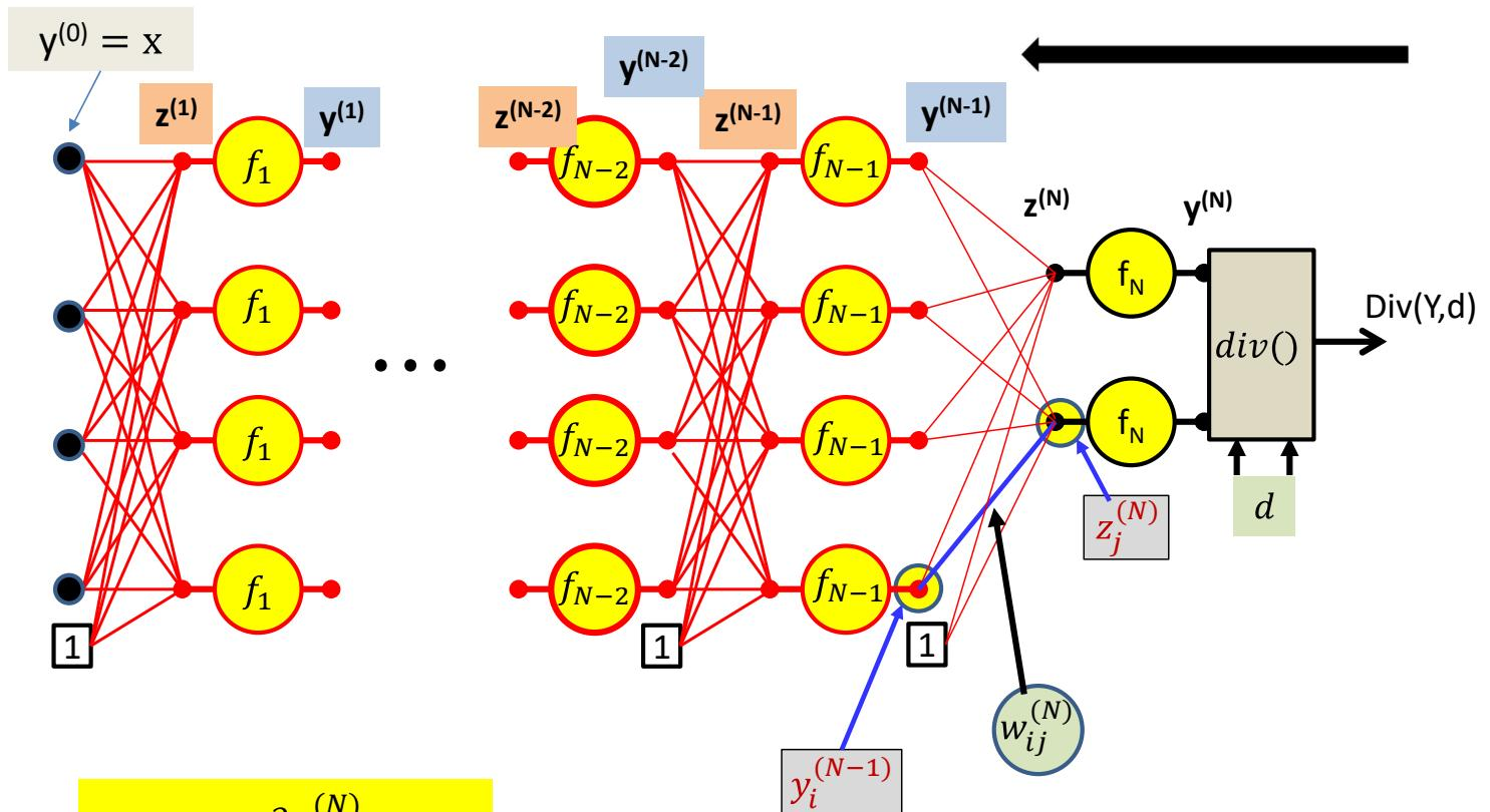
$$\frac{\partial Div}{\partial w_{ij}^{(N)}} = \frac{\partial z_j^{(N)}}{\partial w_{ij}^{(N)}} \frac{\partial Div}{\partial z_j^{(N)}}$$
