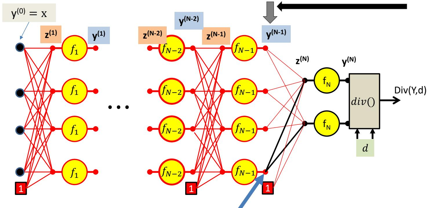
$$\frac{\partial Div}{\partial y_i^{(N-1)}} = \sum_j \frac{\partial z_j^{(N)}}{\partial y_i^{(N-1)}} \frac{\partial Div}{\partial z_j^{(N)}}$$
