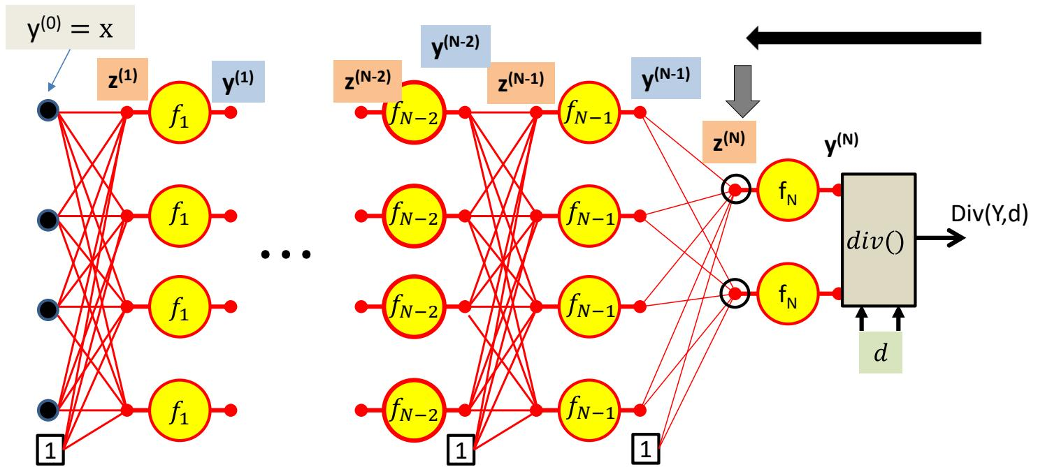
$$\frac{\partial Div}{\partial z_i^{(N)}} = \frac{\partial y_i^{(N)}}{\partial z_i^{(N)}} \frac{\partial Div}{\partial y_i^{(N)}}$$
