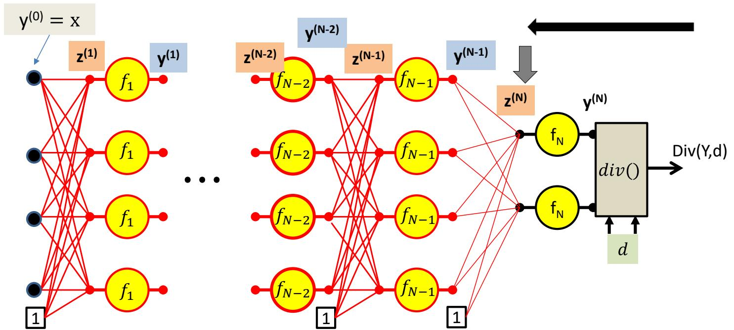
$$\frac{\partial \text{Div}}{\partial z_i^{(N)}} = f'_N(z_i^{(N)}) \frac{\partial \text{Div}}{\partial y_i^{(N)}}$$
