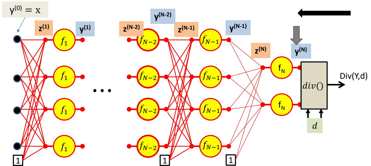
The derivative w.r.t the actual output of the final layer of the network is simply the derivative w.r.t to the output of the network
