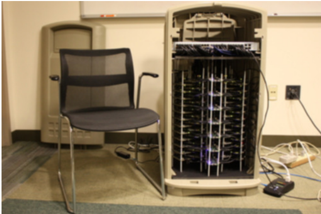
Figure 1. TI PandaBoard cluster used for experiments (photo by Lisa DeLacey)
