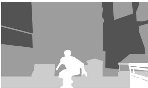
Figure 13: Simplified Z-buffer of the image.
