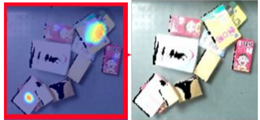
Grasping (think of each pixel as an arm of the bandit, learn which pixel results in grasp)
