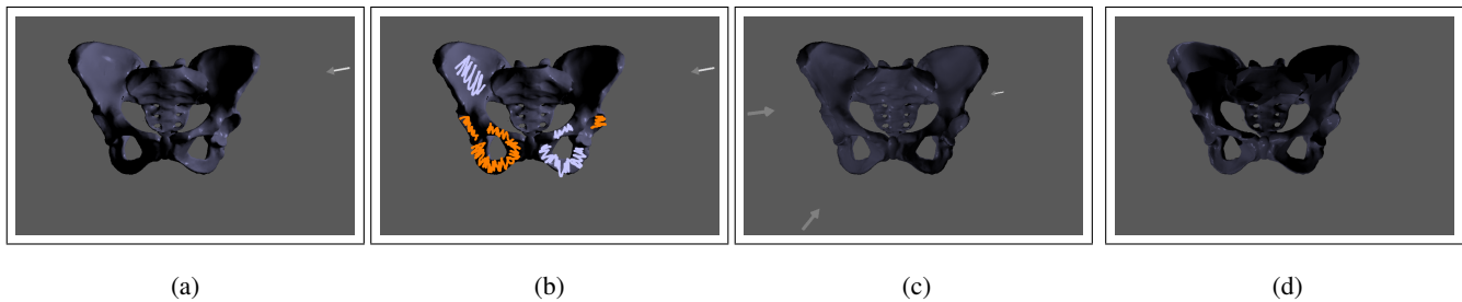
Figure 2: Results: Pelvis. (a) a pelvis model with 50,000 triangles with default lighting. (b) A slightly contrived input is given to switch the contrast between oppositely lit lower cavities. (c) the system realizes this input by adding two lights and moving the existing one. Notice how one lower cavity is highlighted while the other remains dark. (d) the final ray-traced output.
