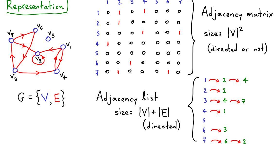
Adjacency matrix size:  $\Theta(V^2)$ directed or not Adjacency list size:  $\Theta(V+E)$ Same for "dense" graphs, i.e. Adj. list uses less space for "sparse" graphs · How much time to ...
